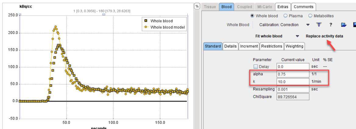
Next, enter the values for **alpha** and **k** determined with the calibration experiment. The dispersion corrected blood activity is shown as the **Whole blood model** curve. The **Delay** parameter represents the delay of the corrected curve relative to the blood arrival at the target tissue, as usual.
